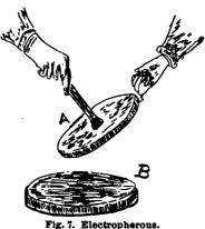
contact with the vulcanite; then lifting the plate by its glass handle, a very strong spark can be drawn from the plate, and this can be many times repeated without a repetition of the striking.
